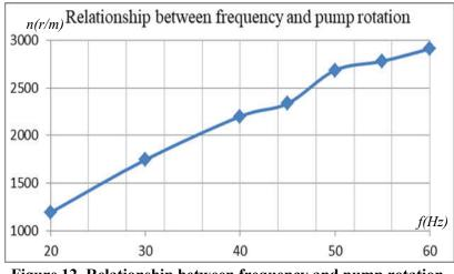
Figure 12. Relationship between frequency and pump rotation
