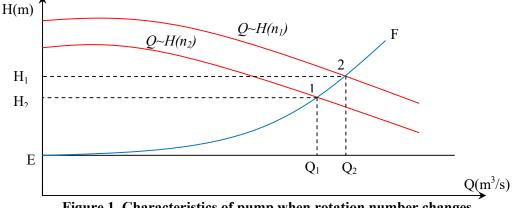
Figure 1. Characteristics of pump when rotation number changes
