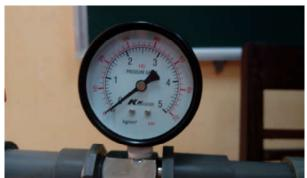
Figure 6. Pressure gauge
