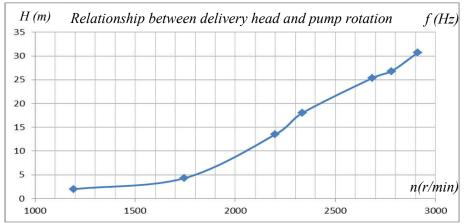
Relationship between delivery head and pump rotation is displayed in figure 13.
