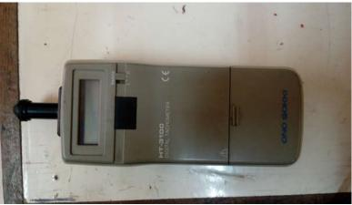
Figure 7. Rotational speed meter HT-3100 of ONO-SOKKI
