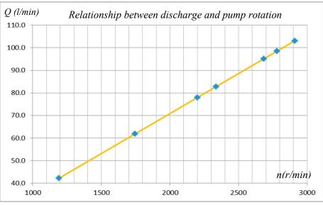
Figure 14. Relationship between discharge and pump rotation
