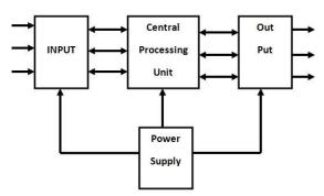
Figure 4. Structure diagram of Programable Logic Controller PLC S7-200
